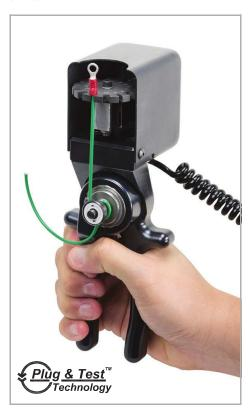
The MR06-200 wire crimp pull sensor is a hand-operated solution for measuring wire crimp pull-off forces. The ergonomic handles and convenient tensioning mechanism make field measurements a breeze for applications up to 1,000 N / 100 Kgf. Squeeze the handles together to increase tension on the sample until a break occurs. The peak force is recorded by the indicator.
